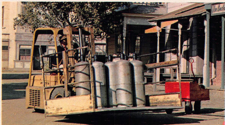
Lift carries butane tanks to scene. Gas was fed through buried hoses.
